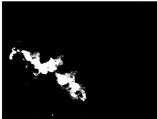
Fig. 6: Segmented image after background removal from the sequence of thermal images during monitoring the ammonia leakage
